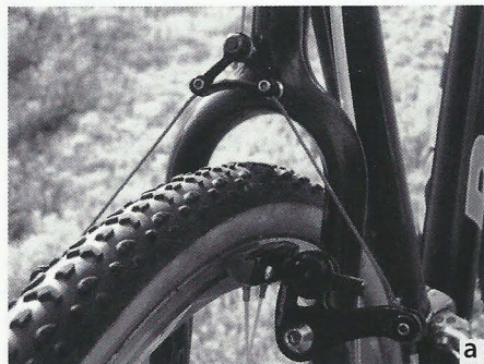
a. Carbon seatstays offer vibration absorption and good mud clearance. b. Aluminum lugs bonded to carbon tubes—a proven construction technique c. Good rear-tire clearance but large lug can collect mud
